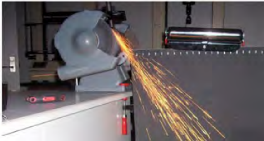
Figure 2: Spark test of a high carbon steel
