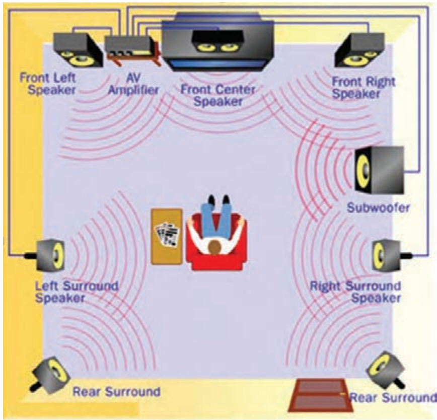
7.1 Surround Sound 2x front speakers 2x surround speakers 2x rear speakers 1x center speaker 1x subwoofer
